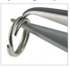
A split ring is useful when extra security is needed to attach charms or to connect a clasp to a piece of jewellery. It works as a doubled up jump ring. To open one you will need a pair of split ring pliers; insert the tip of the pliers into the split ring, and as the gap opens slide on the charm or clasp.
